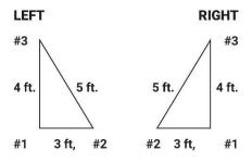
along the twine. Do not remove the #3 pegs yet. Repeat the process at the opposite end of the field making sure the right angles at each corner line up. If you are in doubt, measure the distance from each corner to the opposite corner.
